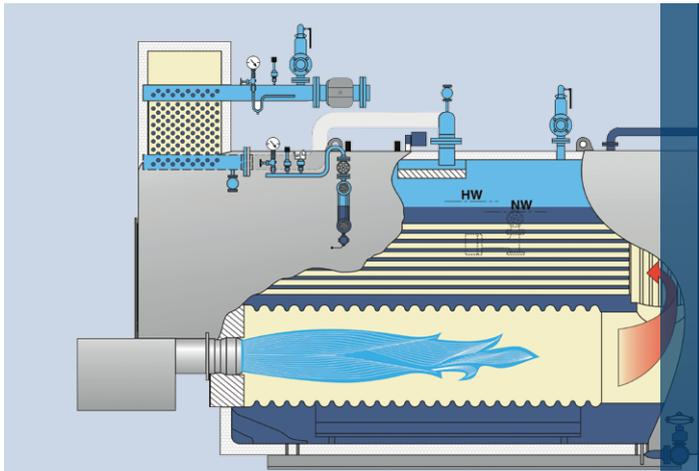
If superheated steam is required instead of saturated steam, a superheater module can be placed on the front reversing chamber. A bypass flap constantly controls the temperature of the superheated steam over a large load range. The smoke tube areas remain easily accessible thanks to the pivoting door of the reversing chamber.
