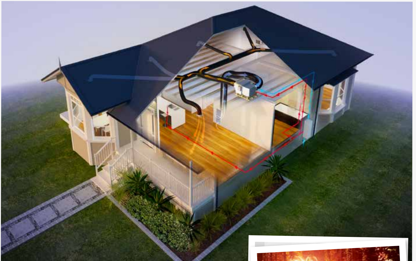
iHeat Central Heating System in the roof cavity
