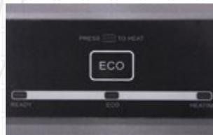
**Eco Mode**, when activated, automatically turns Lazer® Eco off 2 hours after use, helping to reduce power consumption.
