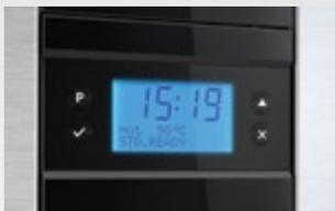
**Timer.** The advanced electronic display (Office & Commercial) also features a seven day programmable timer allowing for the unit to be turned off when not in use. A selectable sleep mode will turn the unit off if it has not been used for a set period of time.
