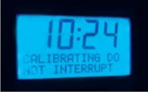
**Auto-calibration.** Rheem have designed a unique auto-calibration function. This means the On-Tap unit can be installed at any altitude and will automatically calibrate to 2°C below boiling point. This ensures you always get the hottest water possible.
